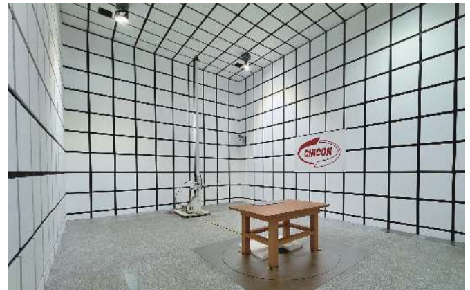
3M Compliant Semi-Anechoic Test Chamber
