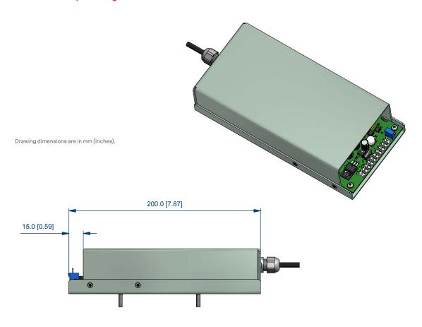
MOUNTING: 2 OFF M4 STUDS; LENGTH AND POSITION AS SHOWN DIMENSIONS mm (in)
