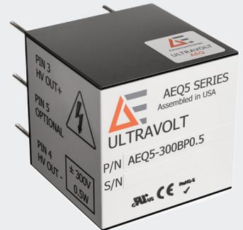
The UltraVolt® AEQ series of ultra-miniature UL approved isolated single or dual output DC to DC converters supply up to 600 VDC at 0.5 or 1.25 Watts of output power from an input voltage of +5 or +12 VDC. The small size of the units and ease of control make the AEQ series optimal for hand-held devices, portable equipment, and other small high-voltage projects.
