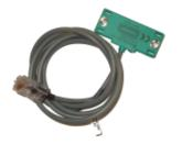
The fuel sensor uses a light barrier to measure whether the level of the fuel cartridge is above or below the position of the sensor and passes on this information.
