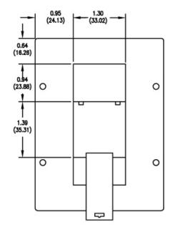
$\begin{array}{l} \mbox{Mechanical Tolerances} \\ \mbox{X.XX} : \pm 0.020 \ \mbox{inches} \ (.51mm) \\ \mbox{X.XXX} : \pm 0.005 \ \mbox{inches} \ (.127mm) \end{array}$
