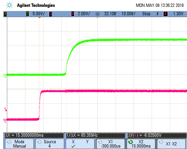
Turn-on transient at zero load current (10 mS/div, Top Trace: Vout, 5V/div; Bottom Trace: ON/OFF, 2V/div)
