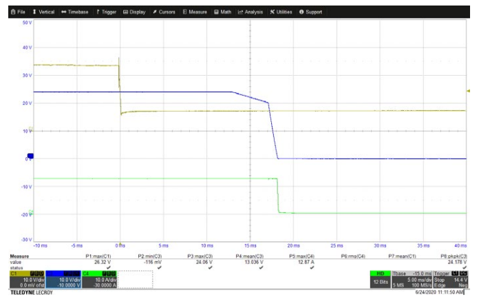
Hold Up/Interruption Time: Measured hold up time with 24Vo/300W Ch1: Vin Ch3: Vout Ch4: Iout (NOTE: for models with Hold Up option)
