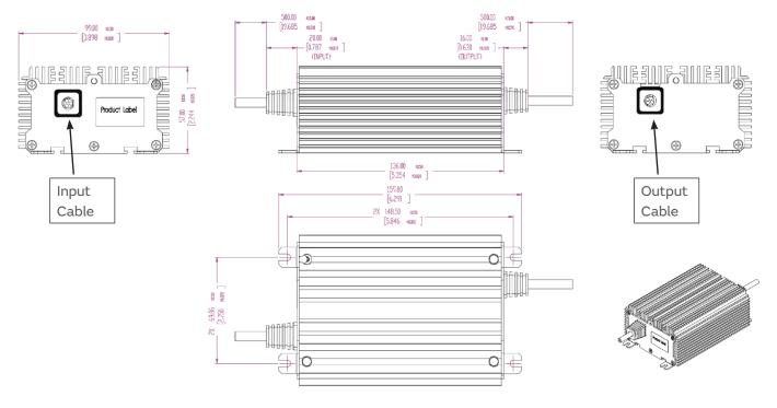
NOTES: 1. THE DRAWING IS A GRAPHIC REPRESENTATION OF THE REAL RODUCT. THE PATTERNS OF FEATURE MAY NOT SHOW ALL FINE DETAILS OR CORRECT PATTERNS. FOR EXAMPLE, THE SCREW FACE PATTERNS OR FAN PATTERNS OR CONNECTORS MAY LOOK DIFFERENT THAN REAL PART. GA USES THIS DRAWING FOR MEASUREMENTS & QUALIFICATION OF DUTGDING PRODUCTS.
