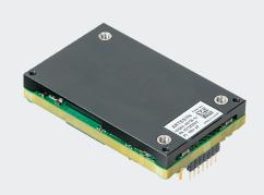
Advanced Energy's Artesyn NDQ900 series quarter-brick non-isolated DC-DC converter provides a single regulated low noise output. It delivers up to 900 W with 12.25 V output voltage and an input range of 40 to 60 VDC. It is designed primarily for use with standard 48 V telecommunications equipment supplies. A PMBus<sup>™</sup> interface is also provided for flexible digital control and monitoring. The main application area is in datacom applications.
