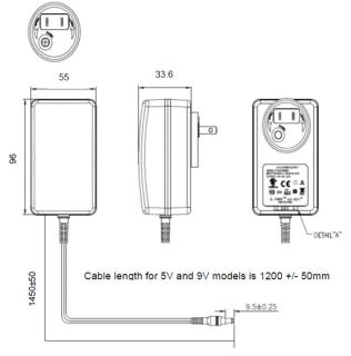
Interchangeable N.A. Blade, 2.5 x 5.5 x 9.5mm barrel connector
