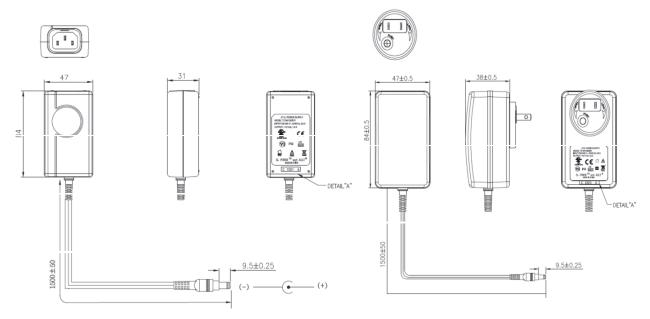
IEC60320C 14 Receptacle, 2 .5 x5 .5 x9 .5mm Barrel Connector
