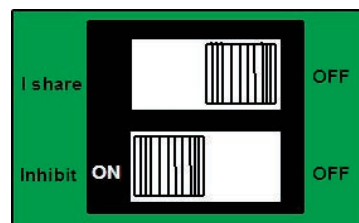
DIP Switch for Current Share & Inhibit/Enable for powerMods XgG to XgT
