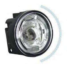
A 70 mm LED fog light of the 2nd generation with the latest LED technology and proven in serial production. Integrated driver with a low power consumption of only 6 W. A very homogeneous light with a light colour of 5950 K and perfect cut-off line together with a very shallow installation depth of only 55 mm. This fog light is homologated for ECE, SAE, CCC and VSCC applications. 2D drawings, 3D CAD data and other data available on request.
