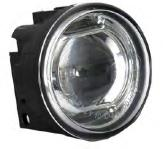
Compact 70 mm LED high beam with a luminous flux measured at 520 lumens and a light colour of 5600 K. Proven in serial applications and perfect in combination with all the 70 mm range. Very shallow installation depth of only 55 mm, therefore particularly suitable for motorbike application, ATV, SSV. This compact high beam has an external driver. 2D drawings, 3D CAD data and other data available on request.
