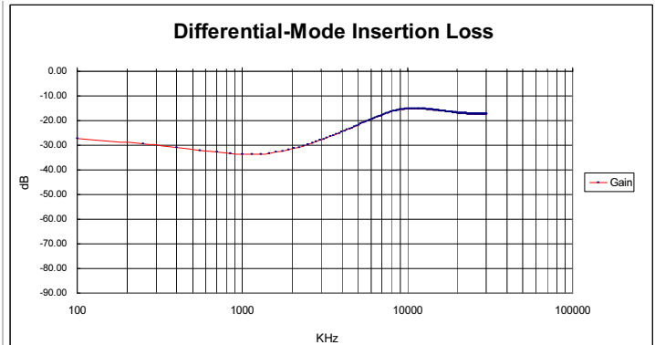
Typical Differential-mode Loss for FM30R080P
