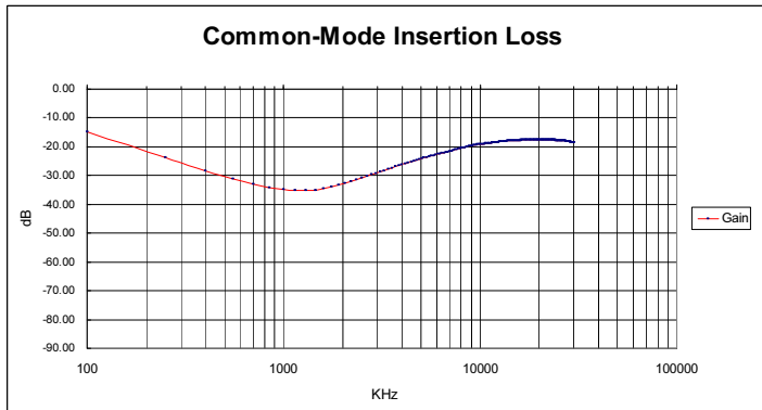
Typical Common-mode Loss for FM30R080P
