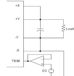
Figure 2 The schematic of output voltage adjusted by using external DC voltage.
