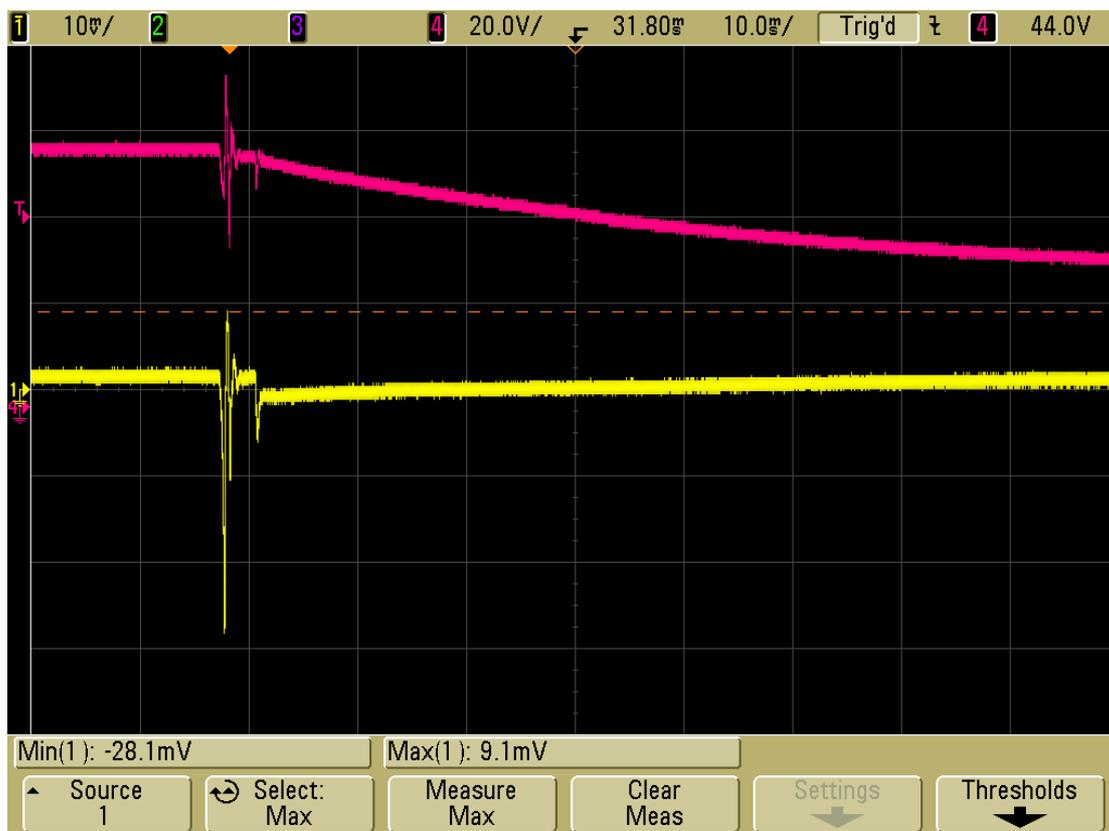
Channel1 (Red) above shows the resultant output voltage spike occurring when the negative current limit is reached, and the output stage goes high impedance. Energy from the load is no longer being dissipated by the power supply and the voltage rises.
