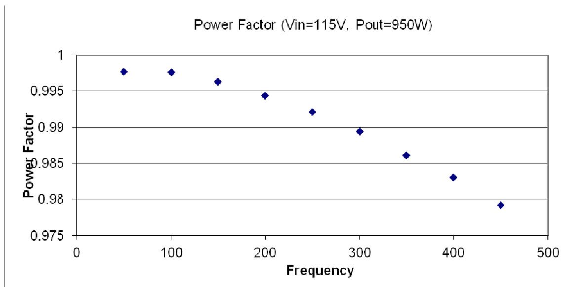
Fig 1: PFC V's Line Frequency, Vin = 115V , Pout = 950 Watts
