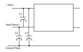
Convertor Z , needs three external components and a ground plane to meet Class B.
