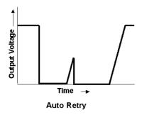
Auto retry is by where the unit will enter a hicc-up mode. This is by where the unit will turn itself off and enter a wait mode. After a certain time the unit will attempt to start itself up again, but will be unable to do so until the fault condition has been removed.
