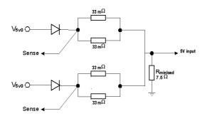
Consider the above set-up. We have two power supplies used in a redundant array. Only one power supply will be on at any given time, and we use Oring diodes to decouple the two power supplies. Because of this there is a drop in voltage across the diode of approx. 0.5 Volts. By sensing the voltage at the destination the converter can automatically increase its output voltage to accommodate for this drop in voltage. The application now has the 5 volts necessary for operation.
