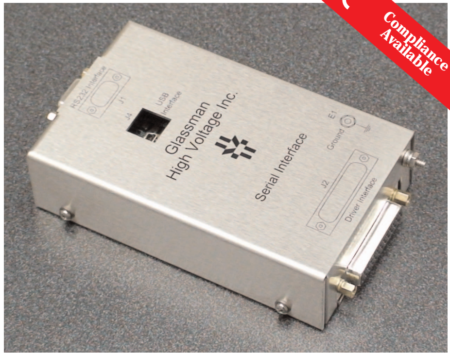
GE9 RS-232 and USB Intelligent Power Supply Serial Interface.
